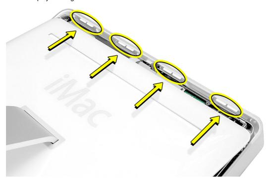
2. Tilt the back cover slightly and align the top edge with the tabs on the housing. Push the two together as you lower the back cover.
